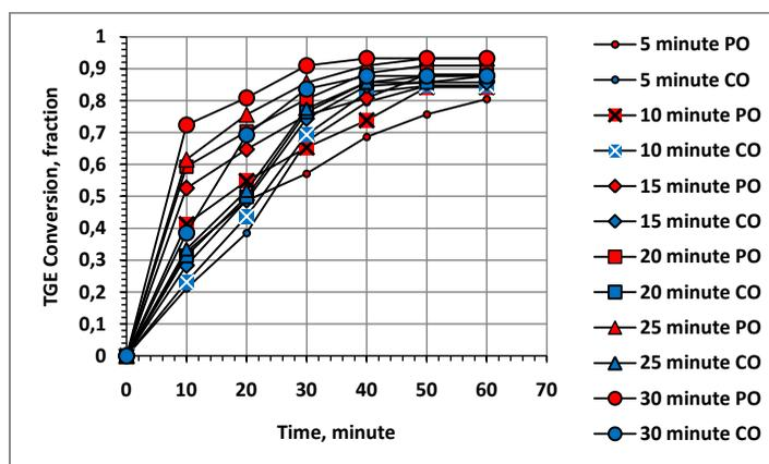
Fig.4: The effect of ultrasonic activation time duration on the Palm and Coconut TGE conversion with the reaction temperature of 70 °C, the MET/TGE ratio of 5 and NaOH catalyst of 1%.
