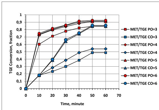
Fig.2: The effect of the MET/TGE ratio and time duration on the Palm and Coconut TGE conversion with the reation temperature of 70 °C, NaOH catalyst of 1% and ultrasonic activation of 30 minutes.
